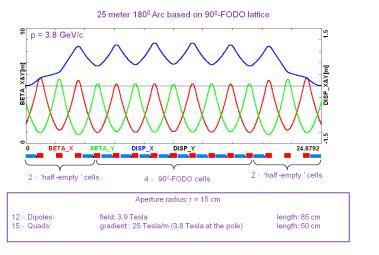
Dispersion in a FODO cell:  $D^{\pm}=\frac{L\phi\left(1\pm\frac{1}{2}\sin\frac{\mu}{2}\right)}{4\sin^2\frac{\mu}{2}}$ . The dispersion has a maximum at the focusing quadrupoles.
