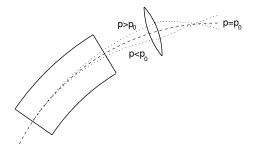
The system introduces a correlation of momentum with transverse position. This correlation is known as **dispersion** (an intrinsic property of the dipole magnets).
