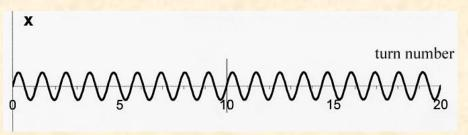
10 turns in the cyclotron for 9 horizontal oscillations  $\nu_r\omega_0\!<\!\omega_0$
