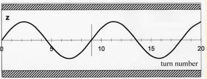
1 vertical oscillation for 9 turns in the cyclotron  $v_z\omega_0<\omega_0$
