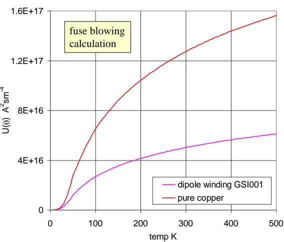
$$\label{eq:Jconstraint} \begin{split} &\text{household fuse blows at 15A,} \\ &\text{area} = 0.15 \text{mm}^2 \ J = 100 \text{Amm}^{-2} \\ &\text{NbTi in 5T} \ J_c = 2500 \text{Amm}^{-2} \end{split}$$
