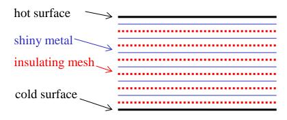
Because radiated power goes as  $\theta^4$  you can reduce it by subdividing the gap between hot and cold surface using alternating layers of shiny metal foil or aluminized Mylar and insulating mesh.
