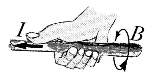
Magnetic field (B) direction around a positive current (I)
