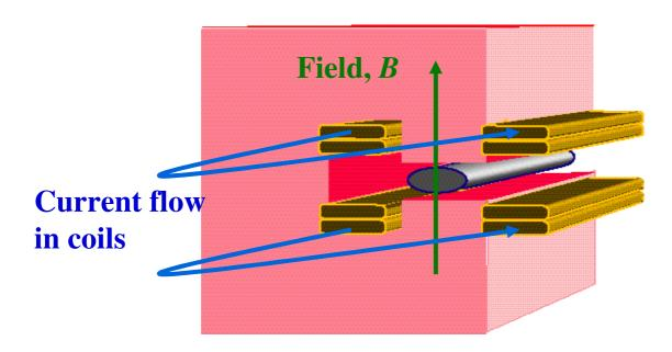
**❖ 'C-shaped' dipole.** Useful for injection, extraction and junctions in transfer lines. Often the poles are inclined to superimpose a gradient on the dipole field.
