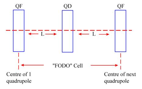
Show that the transfer matrix of a FODO system in thin lens approximation is as follows:
