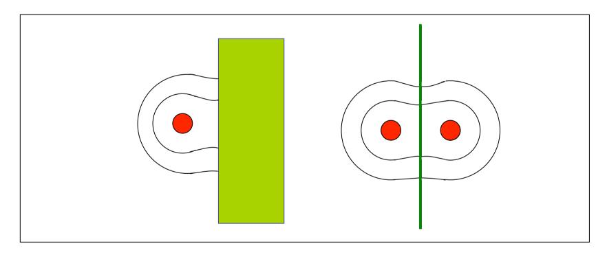
In analogy with the image method we get the magnetic field, in the region outside the material, as superposition of the fields due to two symmetric equal currents flowing in the same direction.
