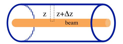
We choose as path a rectangle going through the beam pipe and the beam, parallel to the axis.
