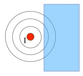
For **ferromagnetic type**, with  $\mu_r >> 1$ , the very high magnetic permeability makes the tangent magnetic field zero at the boundary so that the magnetic field is perpendicular to the surface, just like the electric field lines close to a conductor.
