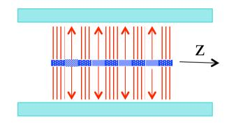
If we take the previous uniform cylindrical beam and enclose it into a cylindric perfectly conducting pipe, the field lines are not perturbed because the electric ones are already radial and then perpendicular to the pipe, and the magnetic ones remain circular. The presence of the pipe does not affect the fields.
