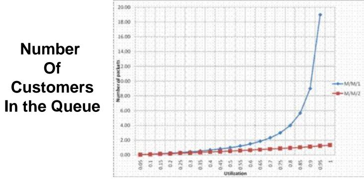
Figure 8. Mean number in System versus utilization for M/M/1 and M/M/2 analytical queue models
