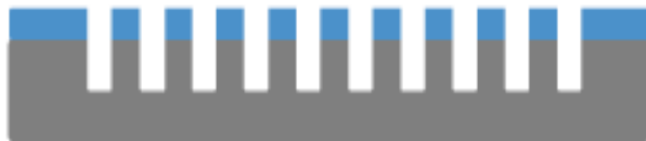
DRIE etching of channels
