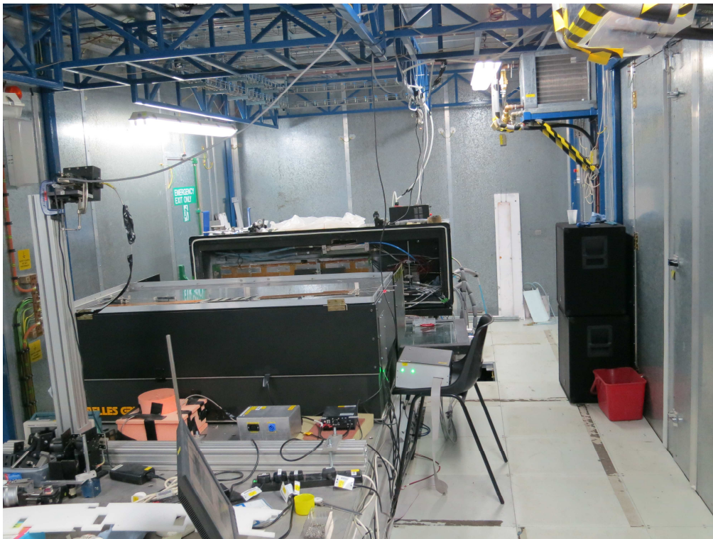
Figure 2: Cold room (with ESPI system in front and thermal test box in rear).
