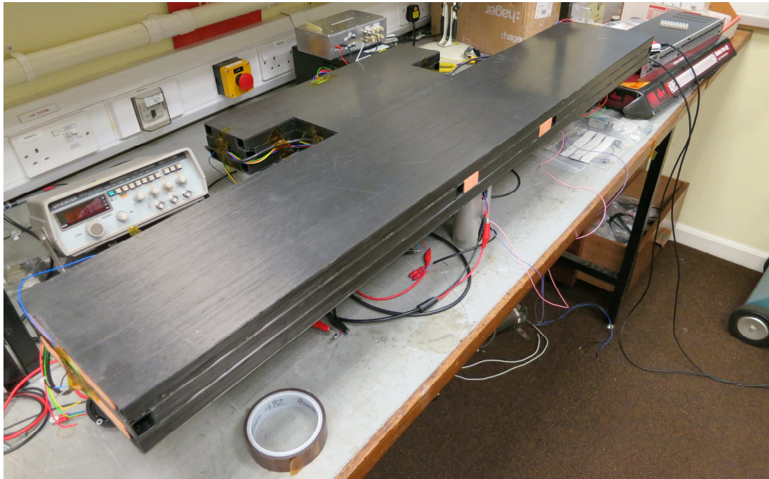
Figure 9: Shaker table for low vibration levels. The table is supported on three points (only front support visible) and excited by a piezo in the front support.
