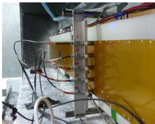
Figure 8: Capacitive sensor system monitoring deformations of ATLAS upgrade stave core prototypes.
