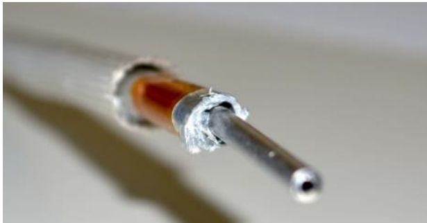
4mm tube with MLI and glass fibre as continuous thermal spacer
