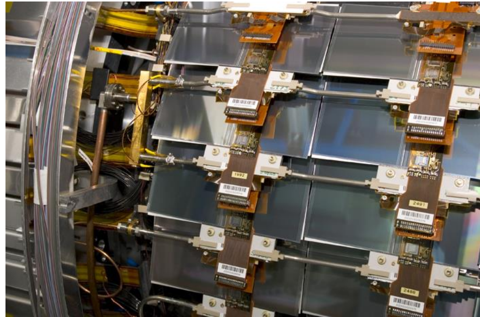
SCT Barrel cylinder showing rows of modules with their services interconnects
