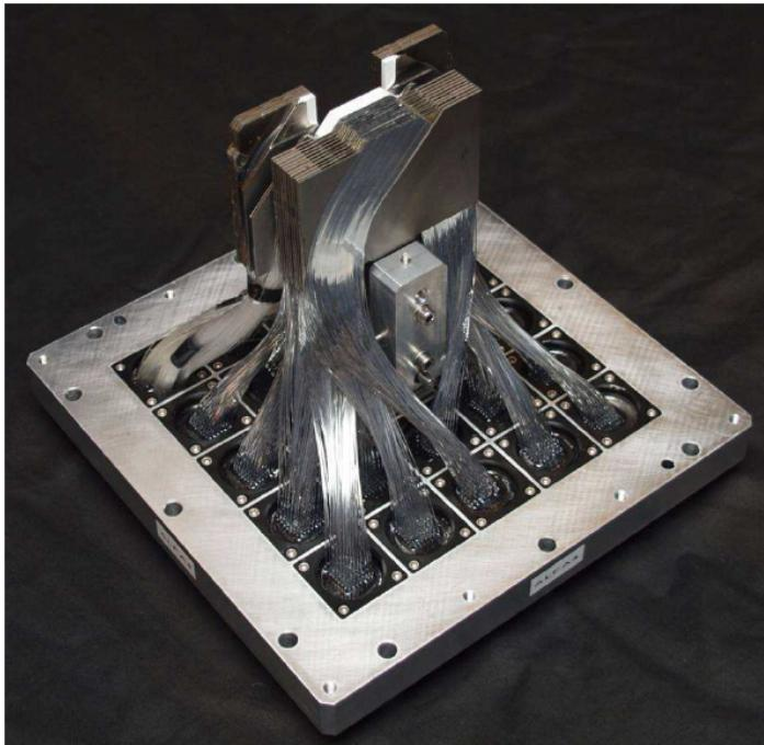
ALFA is a scintillating fibre tracker, 10 double-sided modules with 64 fibres in uv-geometry. Resolution  $\sim 30\mu\text{m}$ .
