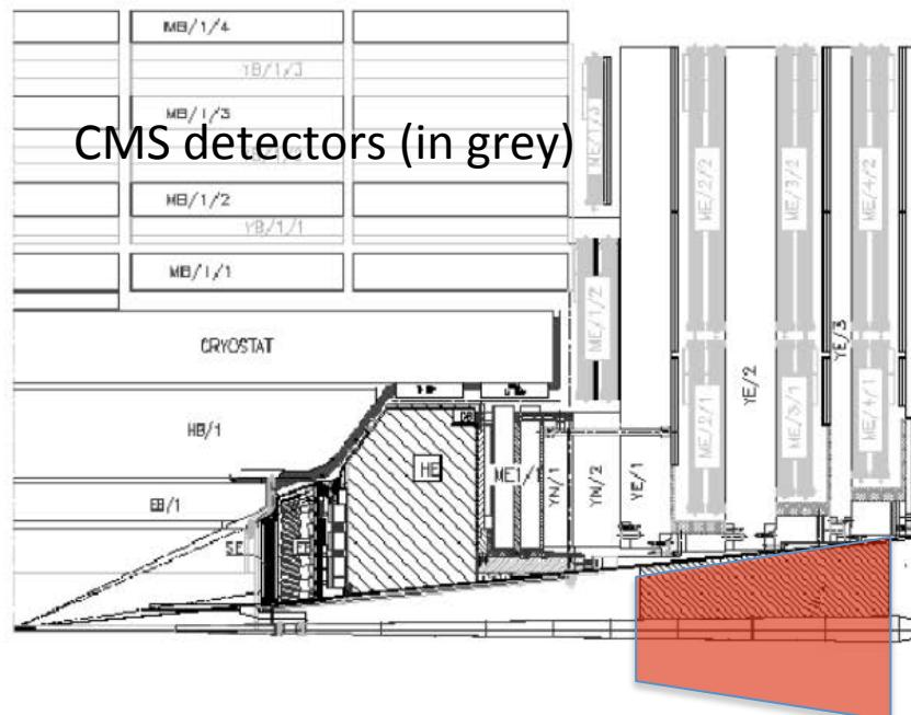
T1 and T2 gas detectors to measure particles from inelastic collisions
