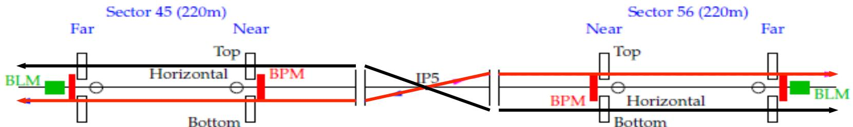
Silicon detectors in Roman Pots to tag elastic and diffractive protons
