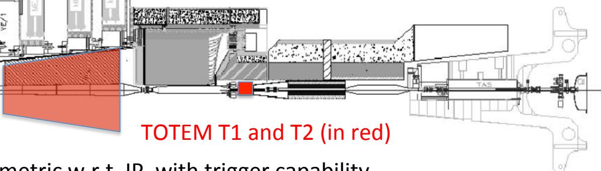
All detectors symmetric w.r.t. IP, with trigger capability
