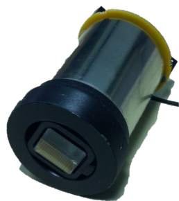
Required assembly of 45 PMT blocks with new active dividers
