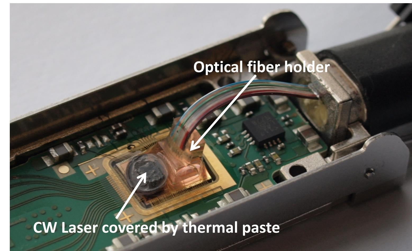
The electro-optical chip, heart of the transceiver, is built using the silicon photonics technology platform developed by Luxtera.
