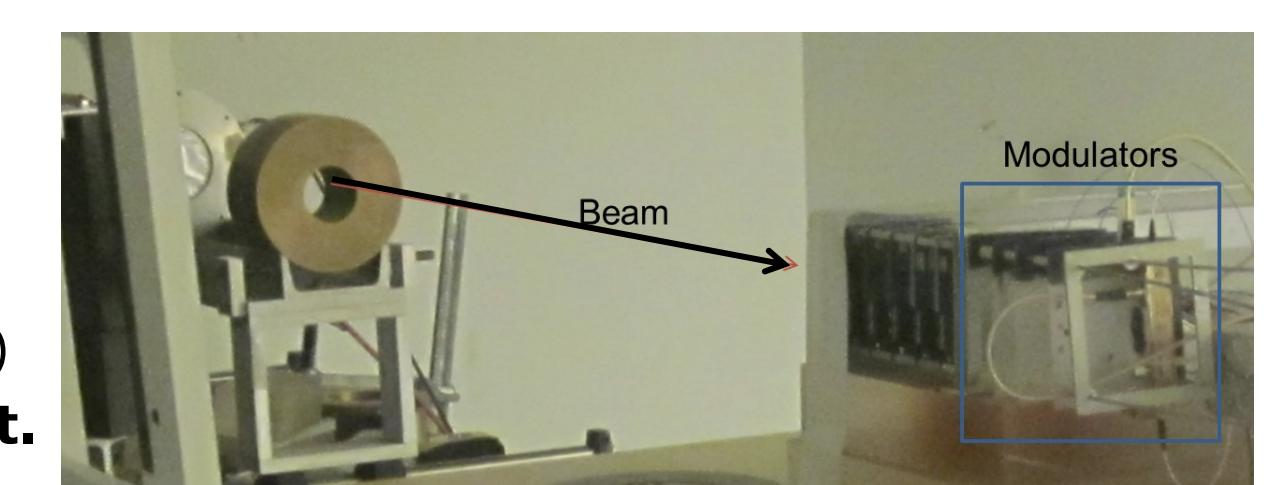
We monitor performance of the transceiver during the irradiation process by recording:
