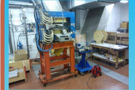
The dipole magnet used for the test (left) and the demo board positioned inside its polar expansions (right). The black rod on which the board is mounted serves for rotating it along the three coordinates
