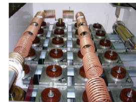
Fig. 16: The SPS extraction PFNs at CERN have 17 cells which are individually 'adjustable'
