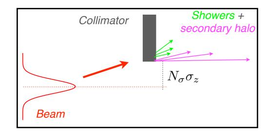
If the "primary" collimator were a black absorber, it would be sufficient to shield the aperture by choosing a gap  $N_{\sigma}\sigma_z$  smaller that the aperture bottleneck ! In reality, part of the beam energy and a fraction of the incident protons escape from the collimator! For "cleaning" what matters is the energy leakage.
