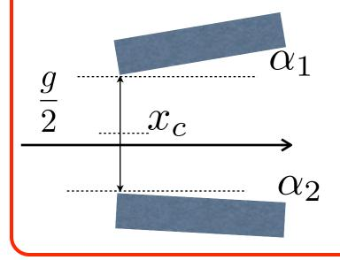
Can apply random errors to collimator geometry. Typical RMS values: Collimator centre =  $50\mu m$ Gap =  $0.1 \sigma$ Jaw tilt angle =  $200 \mu rad$
