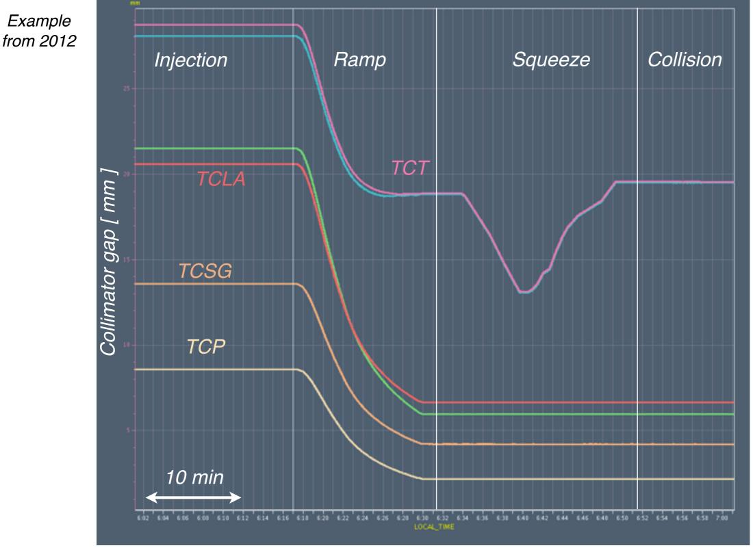
At the LHC, collimator are moved through setting functions versus time.
