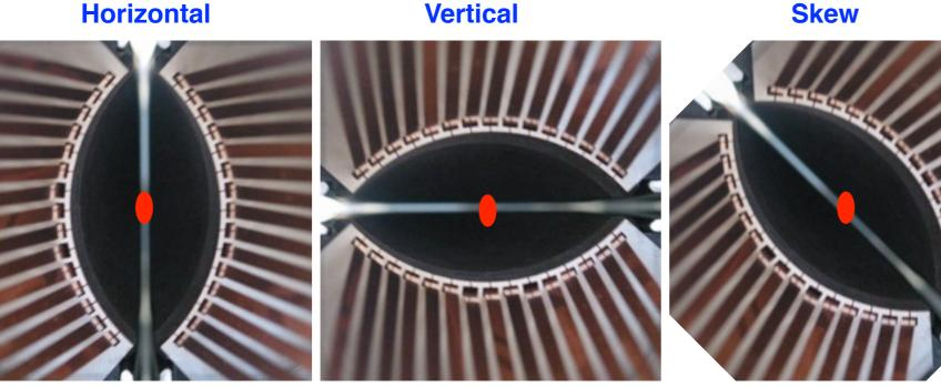
3 primary collimators are needed to protect the machine against transverse betatron losses. Only horizontal collimation for momentum losses.
