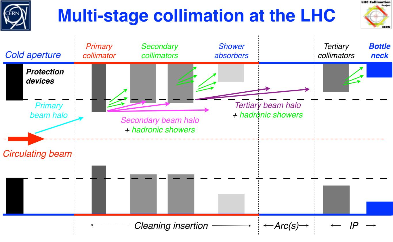
Including protection devices, a **5-stage cleaning** in required! The system performance relies on achieving the well-defined hierarchy between different collimator families and machine aperture.
