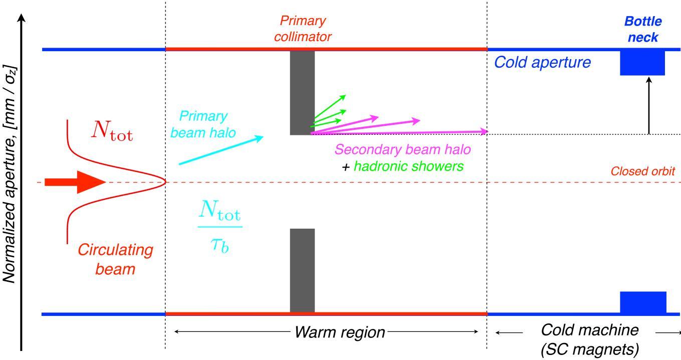
The particles lost from the beam core drift transversally and populate beam tails. Ultimately, they reach the machine *aperture bottleneck*. *Can we stop them with a single collimator that shields the cold aperture?*
