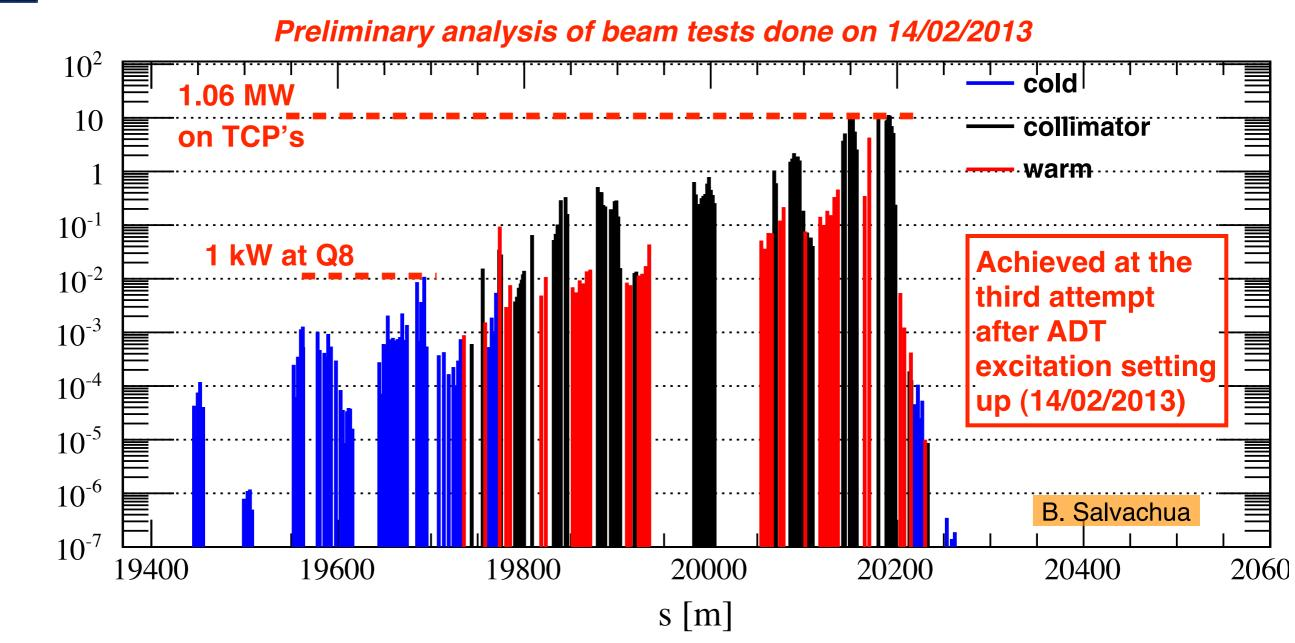
Controlled beam excitation over several seconds: **Peak > 1MW on TCP!** Worsened cleaning by relaxing collimator settings. Achieved 3.4 times the assumed quench limit at 4.0 TeV without quenching!
