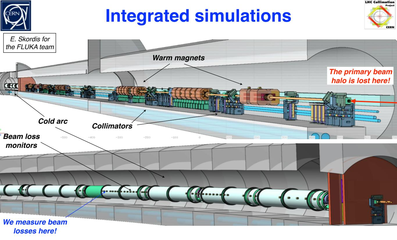
Impressive machine model for energy deposition studies for collimation! This is required to reproduce the details observed in the measurements...
