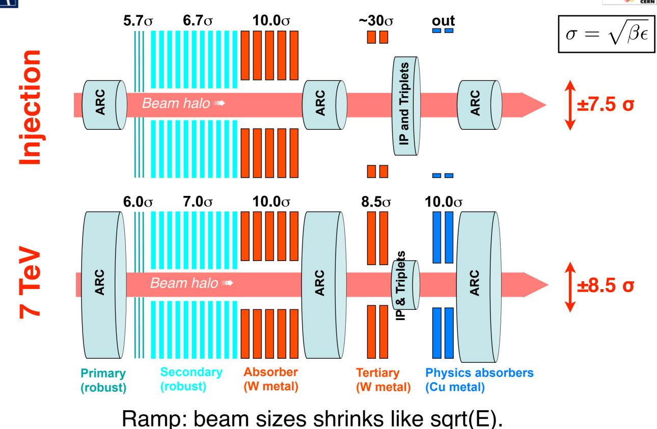
Squeeze optics changes introduce bottlenecks triplet.
