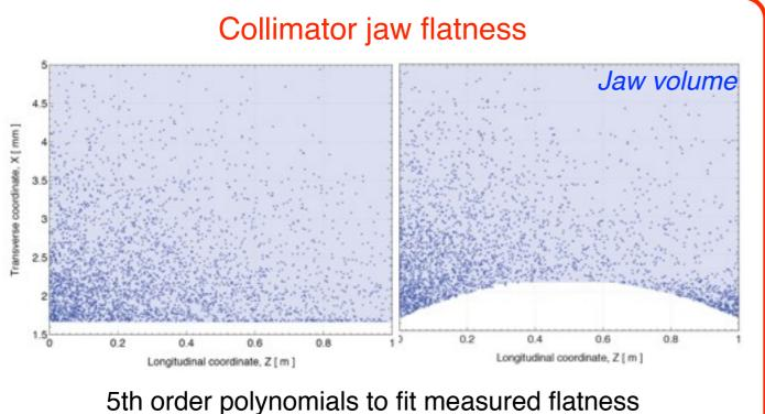
of all Carbon collimators:  $\geq$  40  $\mu$ m
