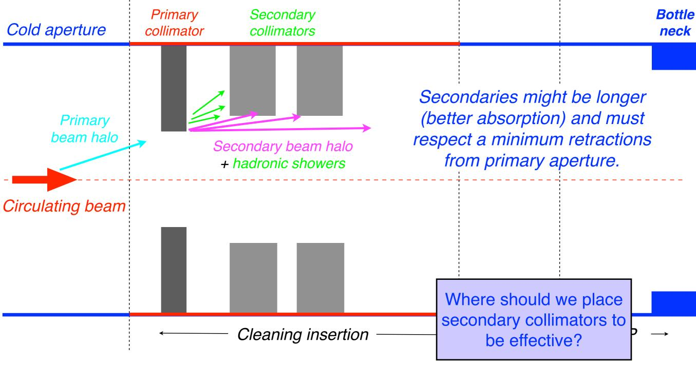
"Secondary" collimators (TCSs) can be added to intercept the secondary halo and the showers that leak out of the primary collimator.
