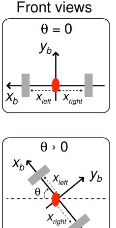
In the LHC, we also have "rotated" collimators that provide collimation in the skew plane. The collimator jaw movement occurs along the skew axis (still 1D movement). Normalized settings are defined for an appropriate effective beam size. Same collimator design for all cases: rotate vacuum tank.
