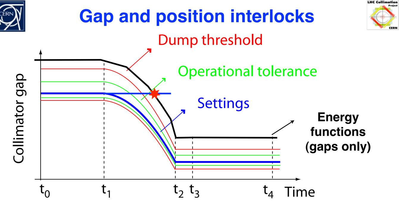
✓ Inner and outer thresholds as a function of time for each motor axis and gap (24 functions per collimator). Triggered by timing event (e.g. start of ramp). "Double protection" → beam interlock AND jaws stopped
