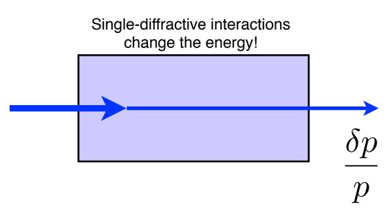
Some protons escape from the collimator with a reduced "rigidity" after loosing energy through inelastic interactions.
