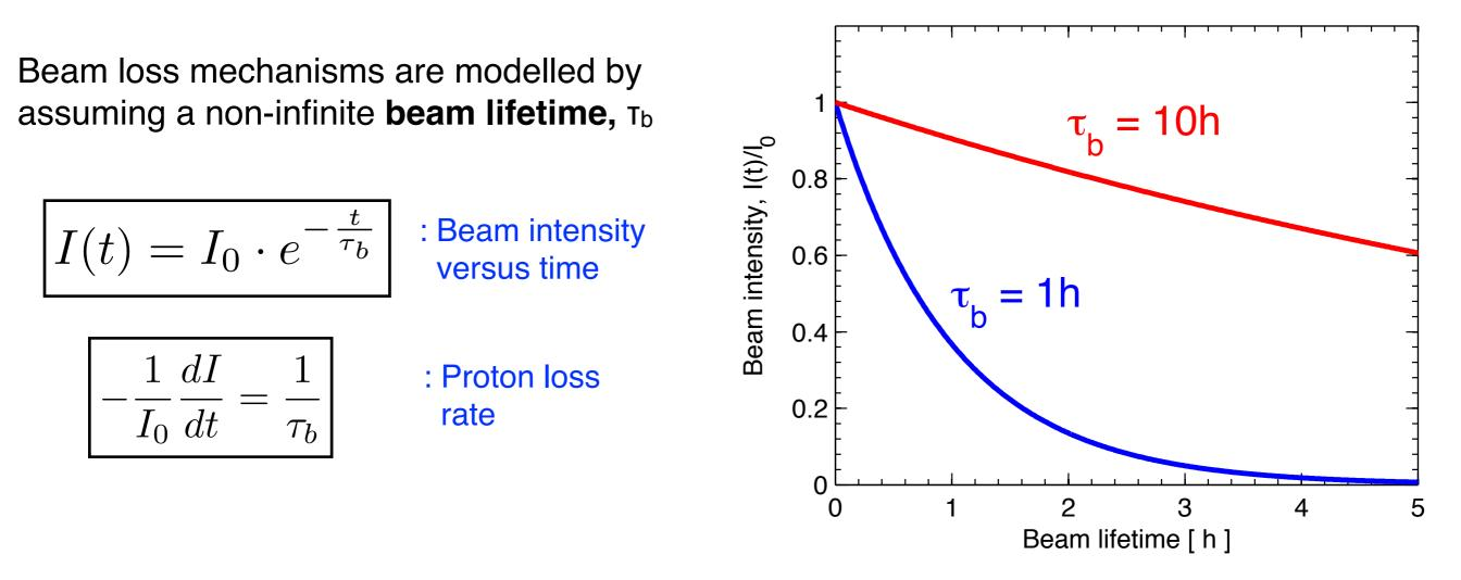
Beam losses mechanisms are characterized by a time-dependent beam lifetime during the machine cycle. This measures the total beam losses that a collimation system must handle.
