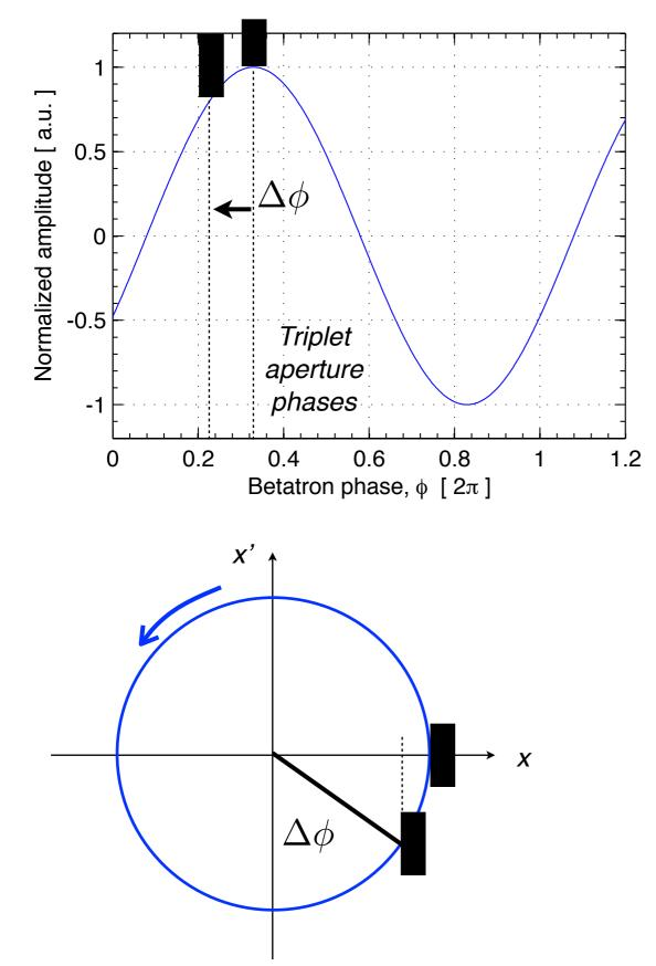
If one cannot install the TCT at the same phase at the aperture bottleneck, equivalent protection levels can only be achieved **closing the collimator to smaller gaps**.
