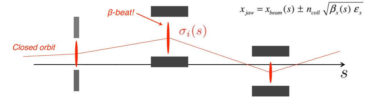
Due to the very small gaps involved, collimators <u>cannot</u> be set deterministically using nominal parameters: alignment errors, orbit imperfections and optics errors cause uncertainties large compared to gaps.
