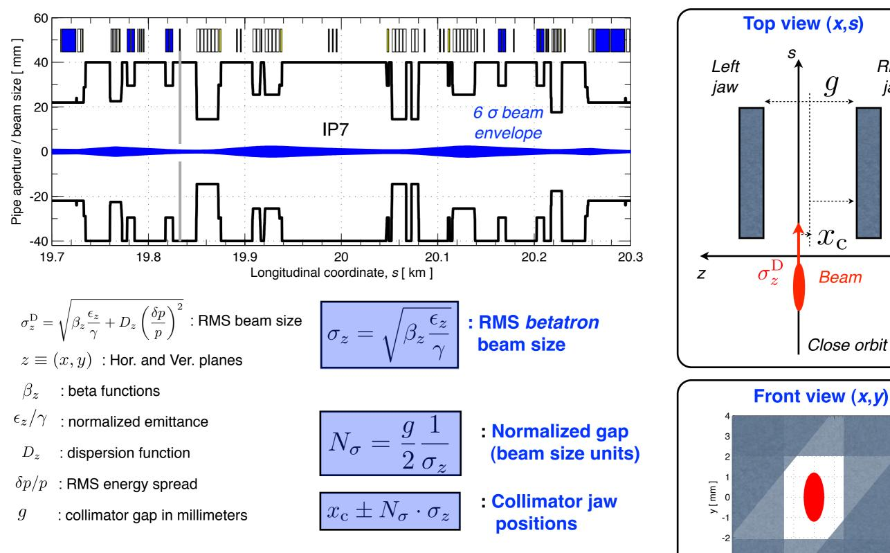
Collimator settings and aperture are expressed in normalized units, using the of local betatron beam size  $\rightarrow$  enable to define the **setting** "hierarchy"!
