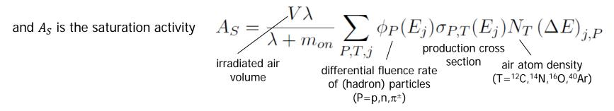
Amount of *activity released into atmosphere all along the irradiation period*  $(t_{on}$  is the time taken by the air flux to reach the release point from the irradiated area)
