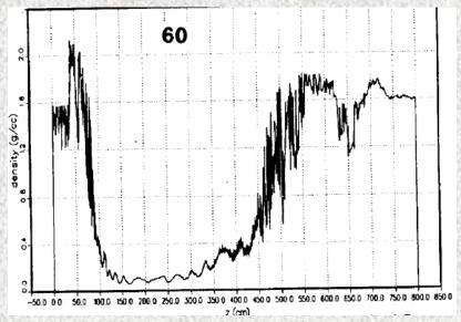
The hole was drilled at the 7 cm/µs penetration rate. Shown is axial density of graphite beam dump in 60 µs after the spill start.
