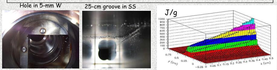
Detailed modeling of dynamics of beam loss (STRUCT), energy deposition (MARS15) and time evolution over 1.6 ms of the tungsten collimator ablation, <u>fully explained what happened</u>.
