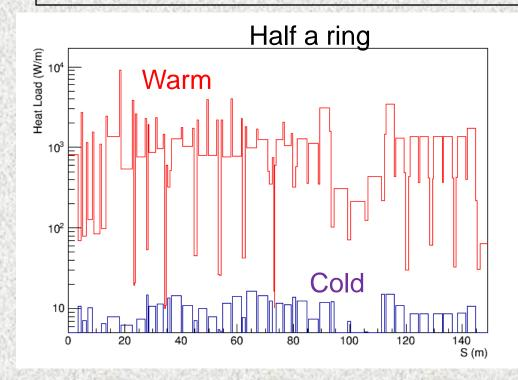
With thick tungsten masks in interconnect regions and inside superconducting magnets, able to reduce average dynamic heat load of ~1 kW/m to the allowable 10 W/m at 4.5K and keep the peak power density in the coils below the quench limit with a necessary safety margin.
