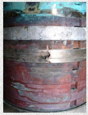
FNAL pbar production target under 120-GeV p-beam (3e12 ppp,  $\sigma \sim$ 0.2 mm)
