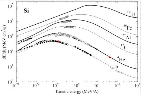
ALi: (i) Lindhard-Sørensen correction (exact solution to the Dirac equation; terms higher than  $z^2$ ); (ii) Barkas correction (target polarization effects due to low-energy distant collisions); (iii) shell correction; Projectile effective charge comes separately as a multiplicative factor that takes into account electron capture at low projectile energies (e.g., z<sub>eff</sub> ~ 20 for 1-MeV/A <sup>238</sup>U in Al, instead of bare charge of 92). JAS, Newport Beach, CA, Nov. 7, 2014
