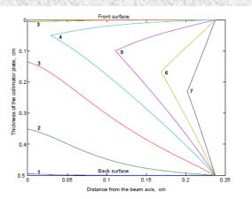
Figure 7: Evolution of the front and back surfaces of the collimator plate at  $t = 0.4_{[1]} - 1.6_{[7]} ms$  with  $\Delta t=0.2$  ms.
