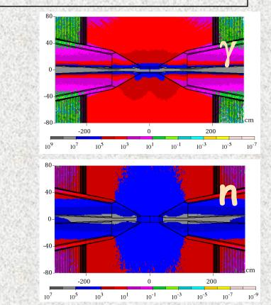
Based on thorough Monte-Carlo, carefully designed massive W-inserts and MDI along with sophisticated tight W-nozzles near IP: ~1000 reduction of heat loads on IR magnets and background loads on detector.
