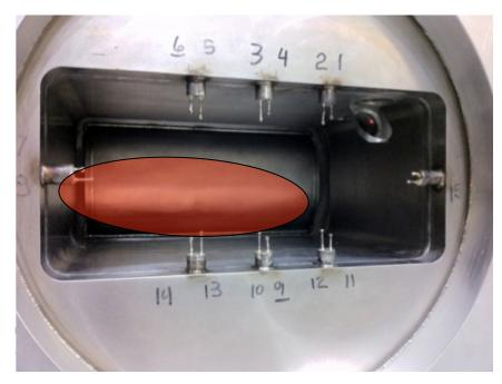
Proton beam window halo thermocouples
