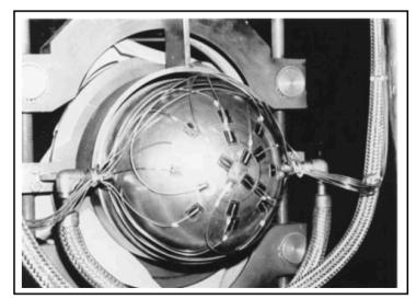
Fig. 2 Outer face (atmosphere side) of the LANSCE double-walled hemispherical beam exit window showing placement of the thermocouples. Note that several spot welds were used to affix the thermocouple pads to the window surface.
