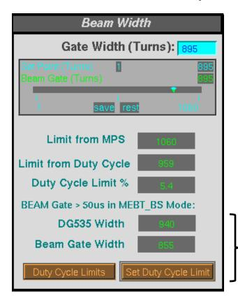
Beam gate width and duty cycle limits, set by operators
