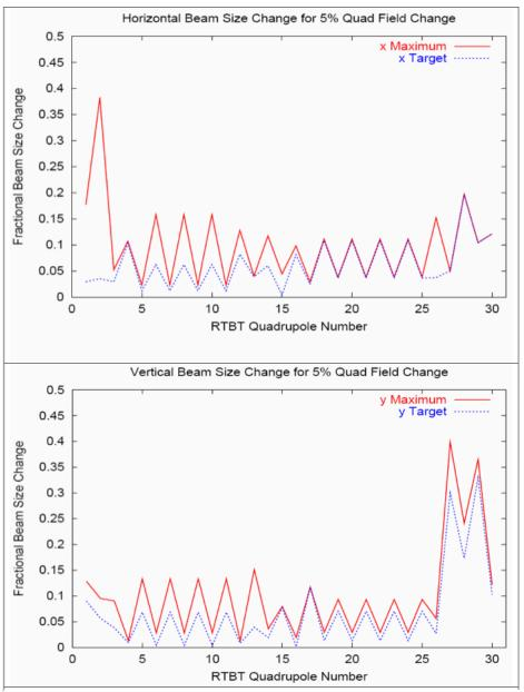
Six of the 19 quad magnet power supplies will cause BLM trips (>0.1% beam loss) before causing dangerous beam parameters at the target
