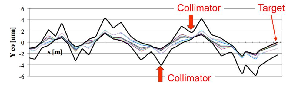
Figure 2: Vertical closed orbit deviation along the RTBT. Thin lines correspond to one kicker misfire. Bold lines are the maximum and minimum closed orbit deviation when two kickers fail simultaneously.
