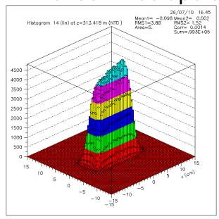
In 2013, J-PARC added two octupole magnets to flatten the beam distribution on the neutron spallation target
