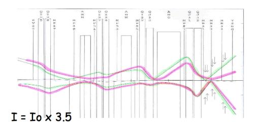
Result: The maximum in the beam density was boosted by a factor of 3.5 resulting in overheating of the center volume inside the target with subsequent damage to some rods and specimens therein.
