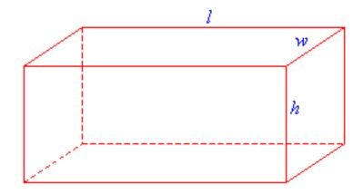
1-second power density =  $(2 \text{ MW})/(2 \text{ cm})/(2 \text{ cm})/(0.75 \text{ m}) = 6.67 \text{ GW/m}^3$
