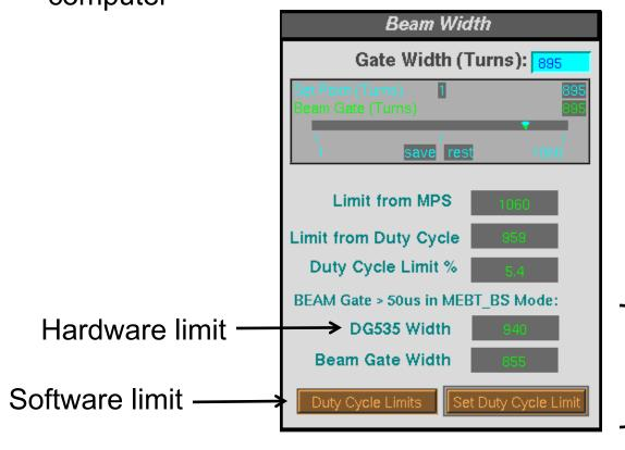
Beam gate width and duty cycle limits, set by operators
