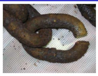
HS broken steel chain from hydrogen embrittlement caused by acidic vapors/condensate from air ionization (MiniBooNE 25 m absorber).
