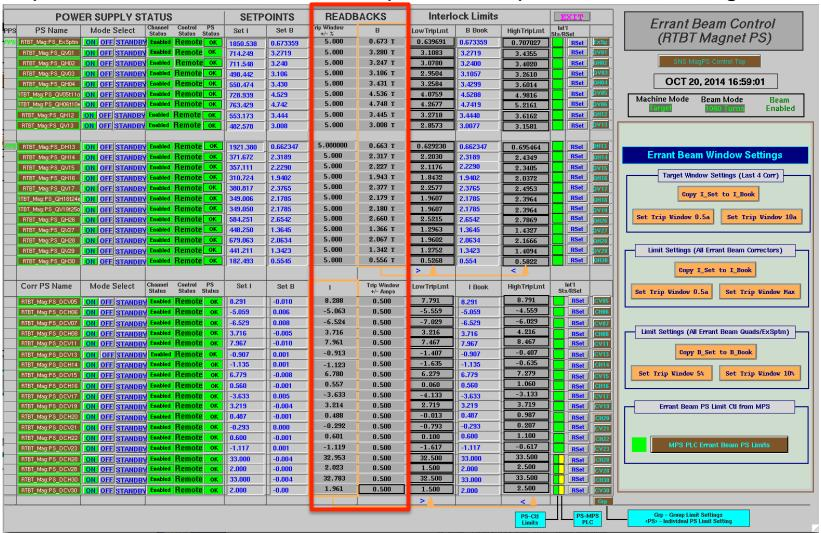
Trip limits set to +/-5% on quads and +/-0.5 A on dipole correctors
