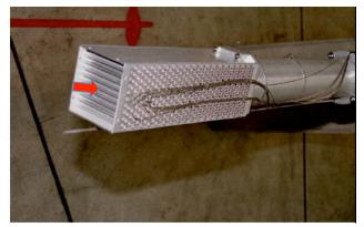
PSI's SINQ target Lead rods, steel tube cladding
