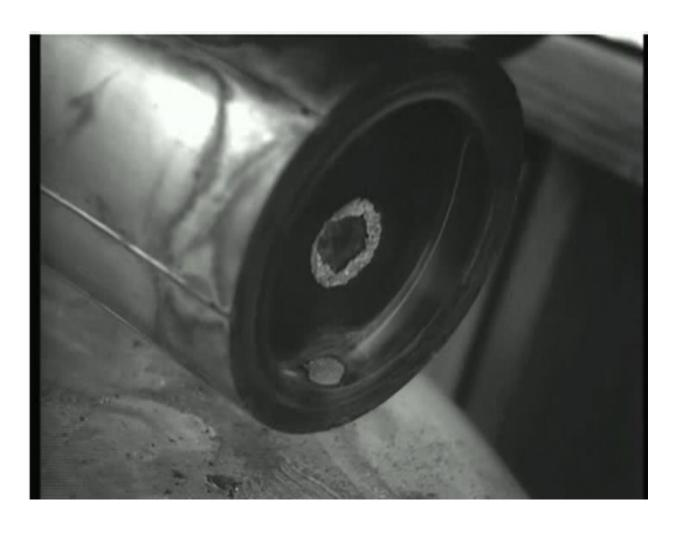
Failure was likely a combination of design error and leaks – possibly analyzed for uniform beam but actual profile gave much higher temperature. Also there was a moderator system water leak which put water in the beam which then disassociated at the high temperature to produce oxygen to attack tantalum grain boundaries.
