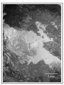
Fig. 12 The crack near both the mechanical center and dose maximum seen from the waterside following removal of some of the deposits
