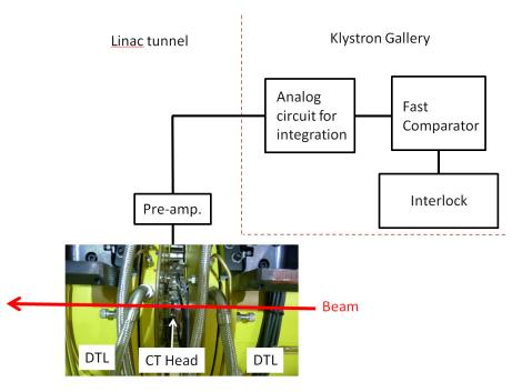
Fast beam current interlock system
