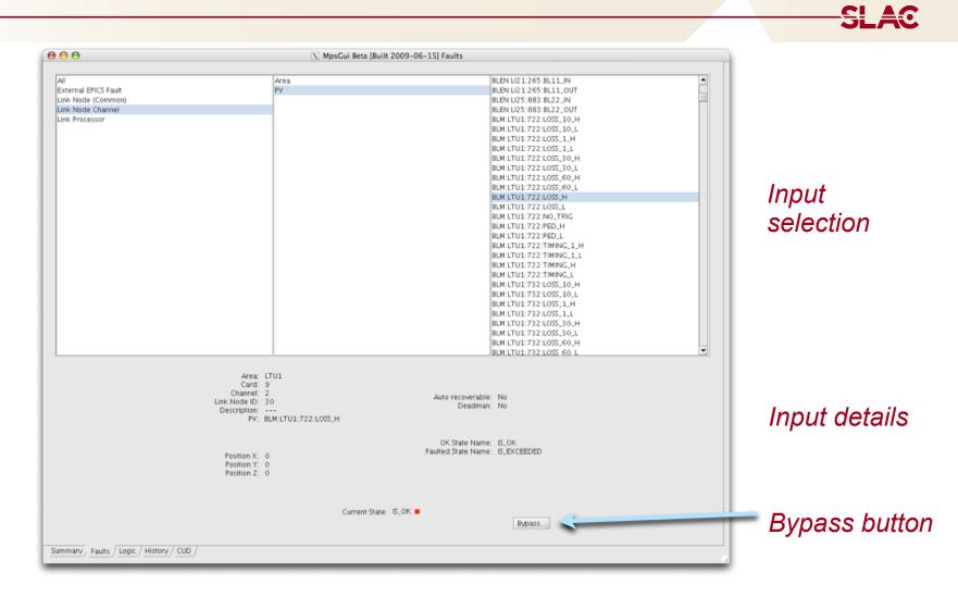
Device faults can be bypassed via an EPICS display by selecting a fault, choosing its bypass state, and supplying a bypass duration.
