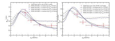
The  $R_{AA}$  in-plane (left) and out-of-plane (right) of D mesons. ALICE data in the 30–50% centrality class are compared to POWLANG results obtained with different transport coefficients (HTL, continuous curves, and L-QCD, dashed curves) and decoupling temperatures ( $T_{\rm dec}$ =170, black curves, and 155 MeV, blue curves).
