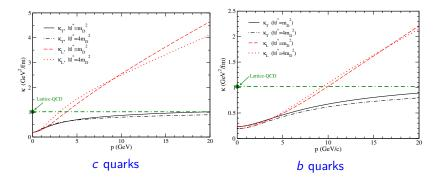
Weak coupling (HTL+pQCD) results for  $\kappa_{L/T}(p)$  are compared to the data provided by the lattice-QCD calculations at p = 0 (and arbitrarily extrapolated at finite  $p_T$ ).
