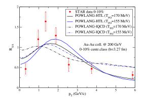
The  $R_{AA}$  of  $D^0$  mesons in central Au-Au collisions at  $\sqrt{s_{NN}} = 200$  GeV. POWLANG results are displayed for the transport coefficients calculated in the HTL framework and constant (extrapolated from L-QCD) and two decoupling temperatures:  $T_{dec} = 170$  and 155 MeV. In all cases heavy quarks are hadronized via recombination with light partons. Theory curves are compared to STAR data.
