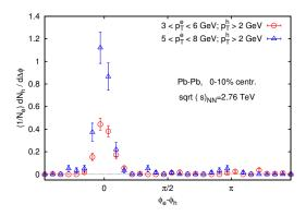
Azimuthal e-h correlations in Pb - Pb collisions at  $\sqrt{s} = 2.76$  TeV for different  $p_T$ -cuts of the trigger particle (e). (Only e's from c's).
