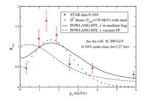
The  $R_{AA}$  of  $D^0$  mesons in central Au-Au collisions at  $\sqrt{s_{NN}} = 200$  GeV. POWLANG results obtained with HTL transport coefficients and a decoupling temperature  $T_{dec} = 170$  MeV are displayed. Also shown for comparison is the limiting case of full kinetic thermalization of Dmesons. Theory curves are compared to STAR data <sup>7</sup>.
