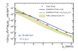
$D^0 p_T$ -differential cross-section in pp collisions at  $\sqrt{s} = 200$  GeV, measured by the STAR collaboration <sup>2</sup>, compared to the predictions of the POWHEG+PYTHIA setup employed in the present work.
