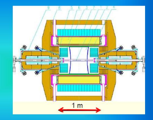
1 – beam pipe, 2 – drift chamber, 3 – BGO calorimeter (680 crystals), 4 – Z–chamber, 5 – CMD-3 superconducting solenoid, 6 – calorimeter LXe (400 liters), 7 – calorimeter CsI (1152 crystals), 8 –iron yoke, 9 – solenoids of VEPP-2000, (not shown) muon range system (scintillation counters) and TOF system.
