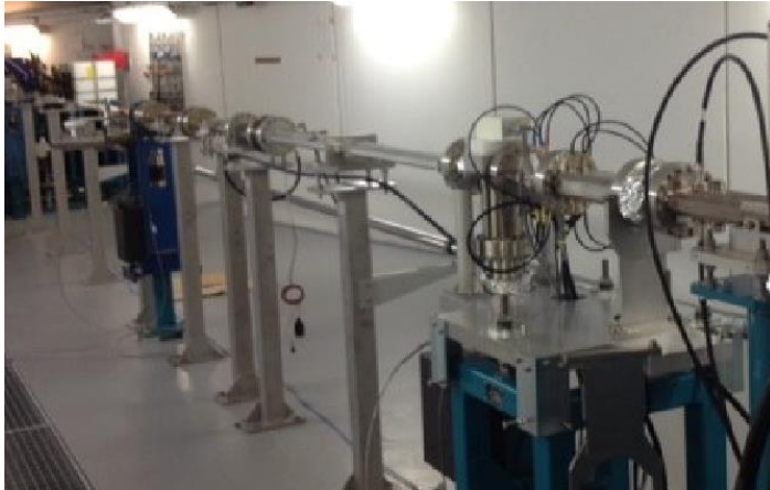
Low gap chamber in a 12 m long straight section in SOLEIL
