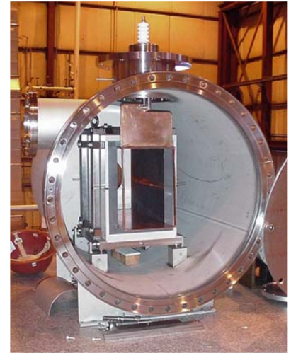
FIG. 7. (Color) SNS extraction kicker: schematic view (left), the kicker in the vessel (right).
