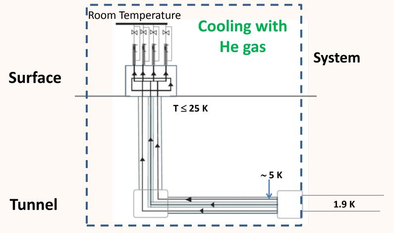
Maximum operating temperature of the cable = 25 K Operation in self-field (B <1 T)
