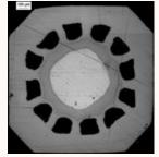
Ni Matrix 12 MgB<sub>2</sub> filaments Cu core – Fe barrier ff  $\sim$  14 %
