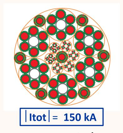
Mass  $\sim$  11 kg/m (880 kg for  $\Delta$ H=80 m)
