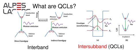
One electron yields > 1 photon Possible to tune the wavelength, operate at room temperature!
