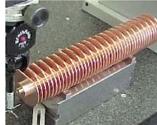
Heat Exchanger (CERN)
