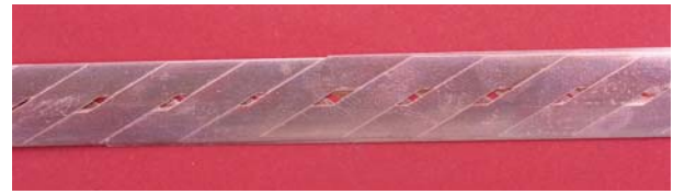
Figure 3: View of the 16 strand ROEBEL assembled coated conductor (RACC).
