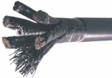
Figure 2: Nb 3 Sn conductor of the TF model coil of ITER made of about 1000 superconducting and Cu strands embedded in a stainless steel conduit.
