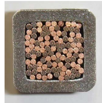
EFDA dipole LF conductor (12.6 x 12.6 mm)
