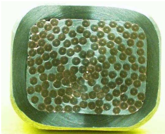
HF Sample 1 (test without solder)
