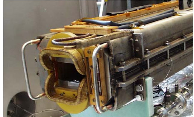
Figure 15: 4KDP6a dipole (connection side).
