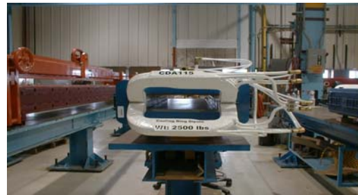
Figure 8: CDA dipole for the HTS and LTS conductor tests
