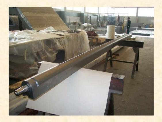
The curved mandrelwas constructed usingwire-sparktechnique.
