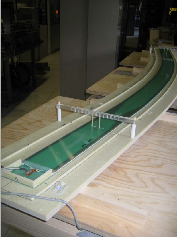
2.5 m curved fluxmeter array for CNAO dipoles
