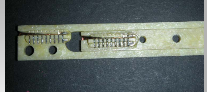
Inset quadrupole-compensated coil for Linac4 PMQs
