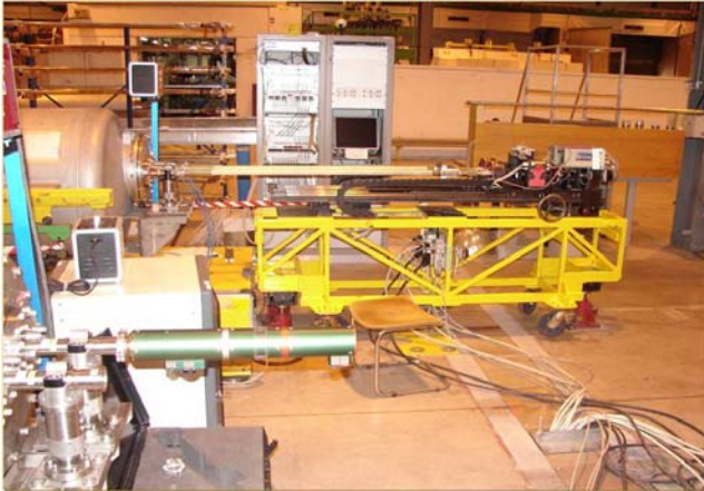
Figure 4: A visual comparison between the Twin Rotating Units, which can be seen in the background while driving two coil shafts inserted in a LHC cryodipoles, and the new Mobile Rotating Unit (in the foreground), directly attached to the anticryostat.
