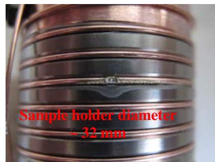
Figure 3: Picture of a round 0.7 mm RRP® strand that had a copper burst during the heat treatment. The wire is mounted on a Ti-Alloy barrels (ITER barrel).
