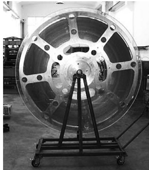
Fig. 2. 1.6 km standard stabilized multifilamentary MgB_2 tape in only one piece.
