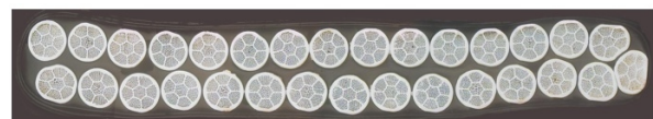
Figure 7: Cross section of a 30 Bi strand Rutherford cable from Nexans (Nexans picture).
