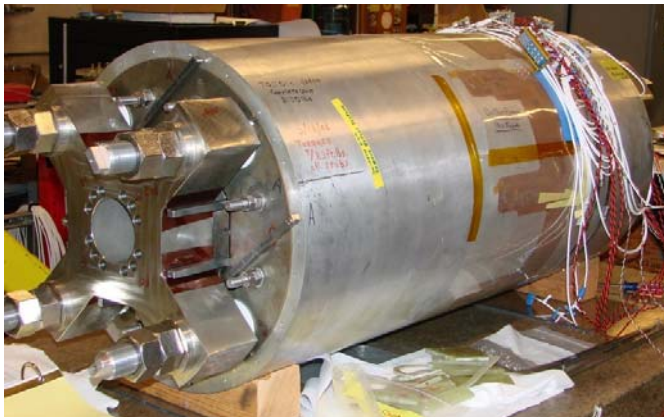
Fig. 1: A ready-for-testing TQS magnet shows the outer aluminum shell, its strain diagnostics, and the yoke. The four large axial rods axially compress the coil-ends, via a thick stainless-steel end-plate.
