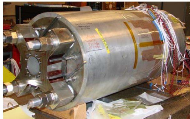
Figure 15. Photo of a completed TQS quadrupole. The four thick rods provide the strong axial support.
