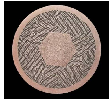
Figure 2: The Nb-Ti strand for ITER model coil PFCI. Strand diameter: 0.73 mm, number of filaments: 2346, filament diameter: 9.8 \mu\text{m} , Cu/non Cu ratio: 1.4, J_c > 2700 \text{ A/mm}^2 (5T, 4.2K) (measured values: 2800\text{-}2900 \text{ A/mm}^2 ).
