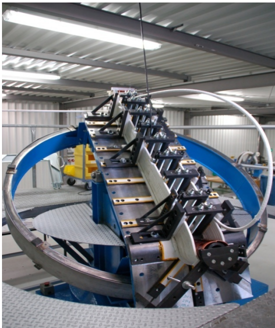
Figure 3: Winding machine with test winding for the Nb 3 Sn dipole.
