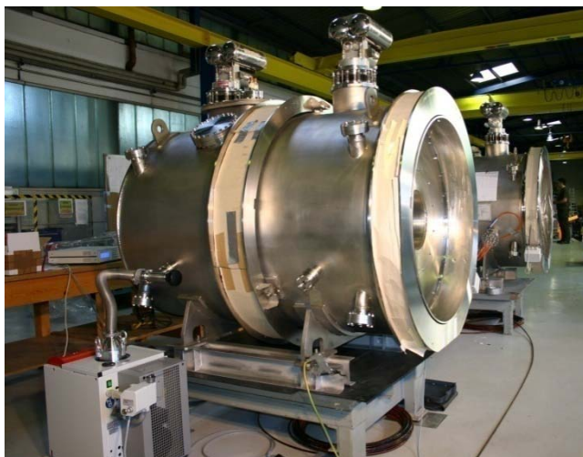
Figure 5: Factory test of a solenoid system for a NSE spectrometer
