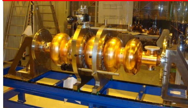
Cell-by-cell tuning system with RF bead-pull and mechanical measurements.
