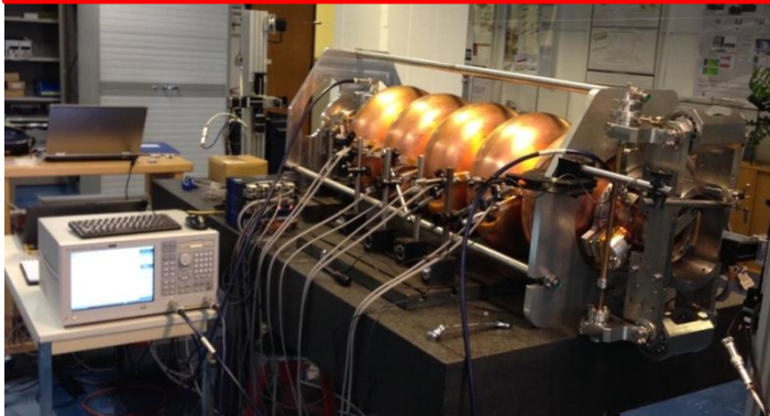
Cavity tuner: measurement of cavity detuning versus mechanical deformation.
