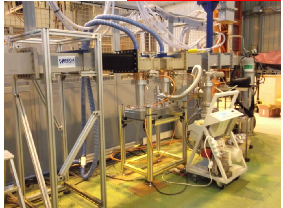
CEA test bench with two SPL cylindrical window couplers, Double Walled Tubes and Test Box cavity
