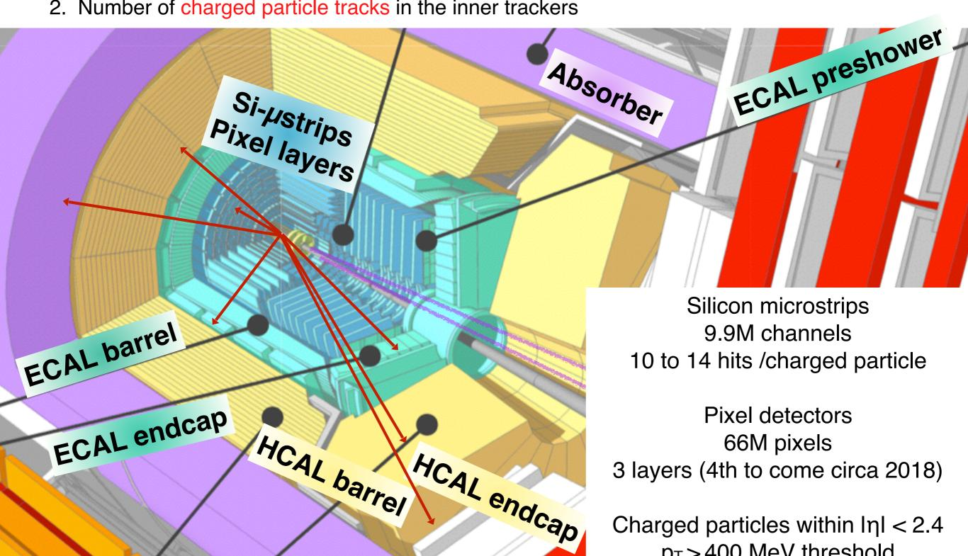
Silicon microstrips 9.9M channels 10 to 14 hits /charged particle
