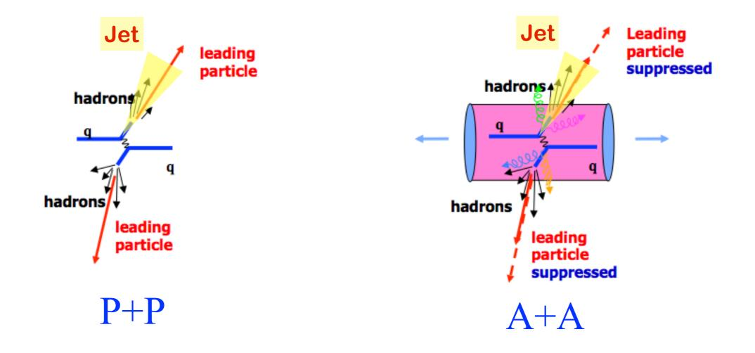
High P<sub>+</sub> leading particles (hadrons)/ jets suppressed in AA collisions w.r.t. PP collisions!
