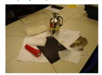
1. PREPARING THE BASE PLATE - If you were not able to get a black metal plate, you have to wrap one side of the metal plate completely with the black electrical tape. This will make it much easier for you to see the "white particle tracks" later on in front of a black background. The bottom will be in contact with alcohol when you run the chamber, so do not use alcohol-soluble tape or glue to attach it. If you have already a black metal plate you can skip to point 2.
