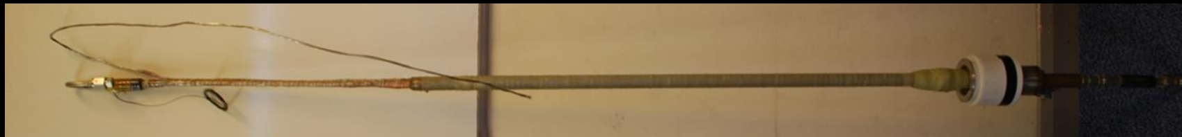
Vapour cooled current lead removed from turret
