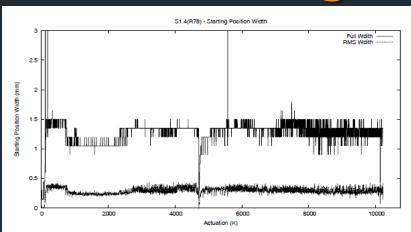
Starting position for the target remained consistent throughout the run.
