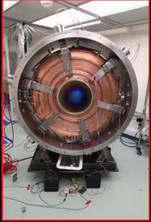
Urgent to start to plan support for MAP test of single-cell cavity in the MTA from the MICE RF group
