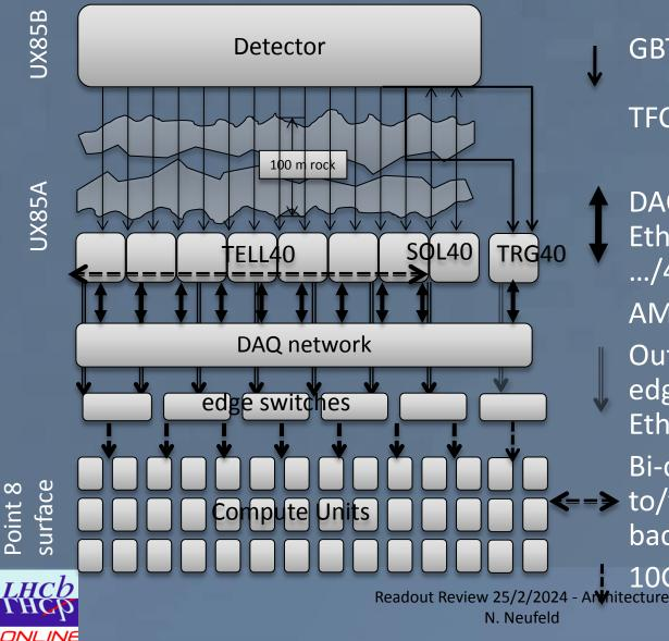
GBT: 4.8 Gbit/s (9000 x) DAQ 3.2 Gbit/s (2400 x) TFC/ECS running over 300 m
